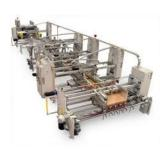
easily handle complex folding and gluing processes inhouse and with increased speed. Steven Lopes, operations manager at Zion, reported that one complicated order that used to take them over seven hours was run in a mere 22 minutes. The new specialty folder gluer allows L&M to handle processes such as auto-lock bottoms, inner partitions, four and six corner trays, and long box styles within a wide range of board grades.
